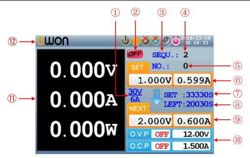
Figure 4-4 User interface in Parallel/Series mode
