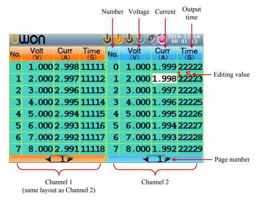
Figure 5-1 Timer Setting Interface in Independent Mode
